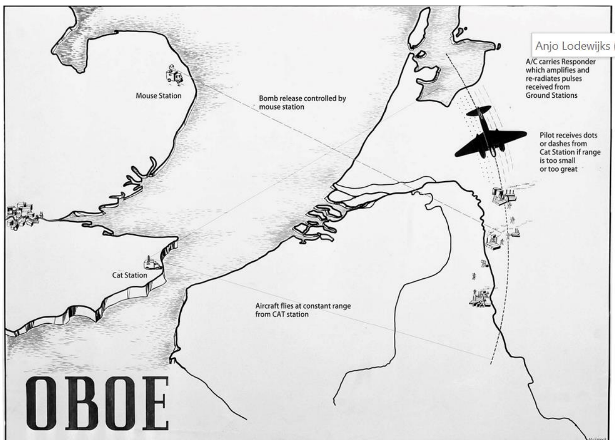
A game of Cat and Mouse. A diagram of the bomber navigation system code-named OBOE.
